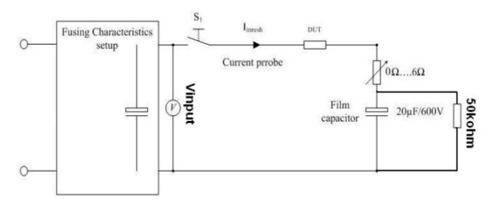
Measure the inrush current (I<sub>inrush</sub>) directly after closing the switch S<sub>1</sub>
